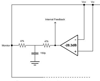
Figure 16: Internal circuitry of the monitor output.
