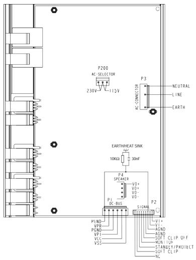
Figure 3: ICEpower500ASP connections
