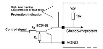
Figure 15: Interface and simplified internal circuit for Shutdown/protect pin.
