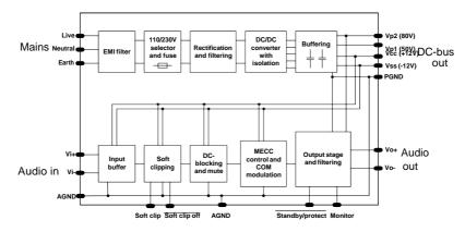
Figure 2: ICEpower500ASP block diagram
