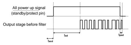
Figure 21: Supply start-up and shut down timing definitions.
