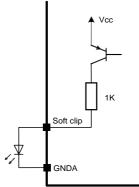
Figure 17: Interface and simplified internal circuit for the Soft clip pin.
