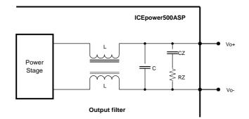
Figure 20: Output filter section with compensating Zobel network.
