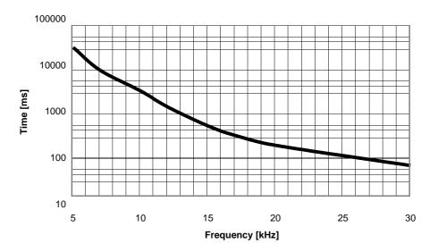
Figure 12: Duration of full output vs. frequency
