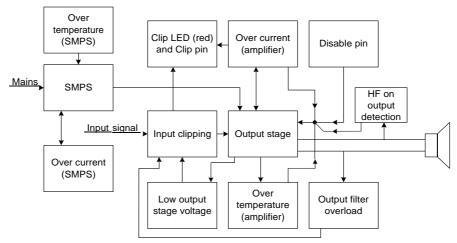
Figure 18: Block diagram of protection features
