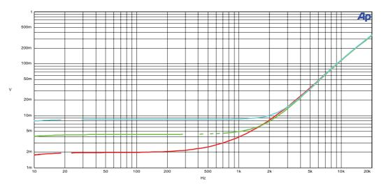
Figure 5: Measured voltage at output terminals while feeding  $1A_{RMS}$  into the output of the amplifier.
