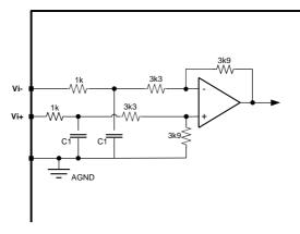
Figure 19: Balanced input buffer.
